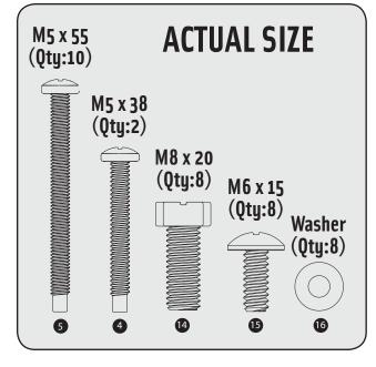
Proper assembly of your new BROIL KING KEG<sup>®</sup> will only require a Phillips head screw driver, a ½ inch or 13mm wrench and a buddy (for lifting). Follow the steps outlined below and it should take approximately 20 minutes to complete. Refer to illustration on page 2 for part(s) identification and placement positions.
