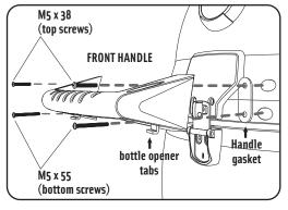
STEP 2: Attach front handle with Phillips head screwdriver. M5 x 55 screws go in the bottom holes with the bottle opener tabs. M5 x 38 screws go in the top holes. Silicone gaskets install behind handle (two places).
