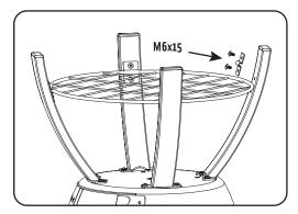
**STEP 6:** Assemble the Hoop to the legs using the Hoop Brackets and the M6x15 screws as shown. Tighten all leg and hoop bracket screws with a screwdriver.
