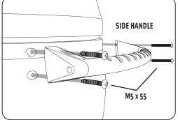
**STEP 3:** Attach side handles (2) using 4 (M5 x 55) screws. Use Phillips head screwdriver. Note the "Bottom"written on the handle and orient down.
