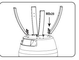
STEP 5: Screw the legs into the threaded inserts in the bottom of the grill using the leg washer and M8x20 screws, (hand tighten only).
