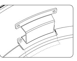
**STEP 9:** Align the notches in the fire bowl with the fire **STEP 10:** Install the Cast Iron Cooking Grate. bowl supports inside the grill (as illustrated).
